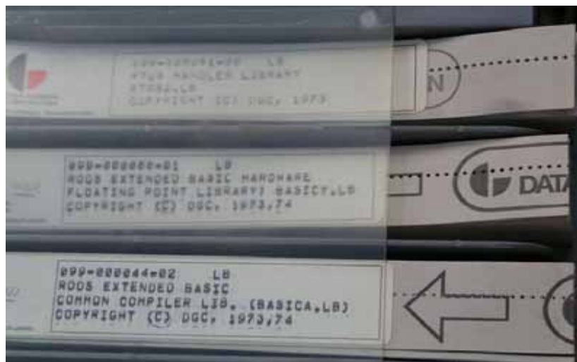
Software on paper tape for the Data General Nova minicomputer.
