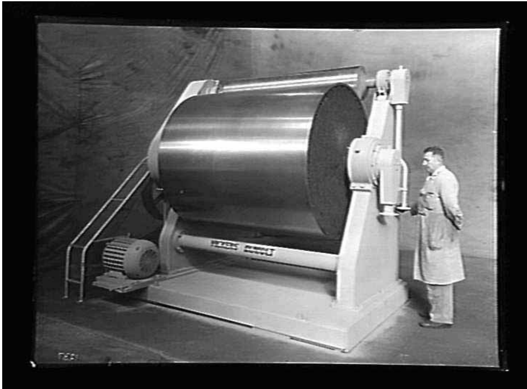
Soap Chilling Drum – molten soap streamed on and chilled soap sliced off like tissue. ca 1956
