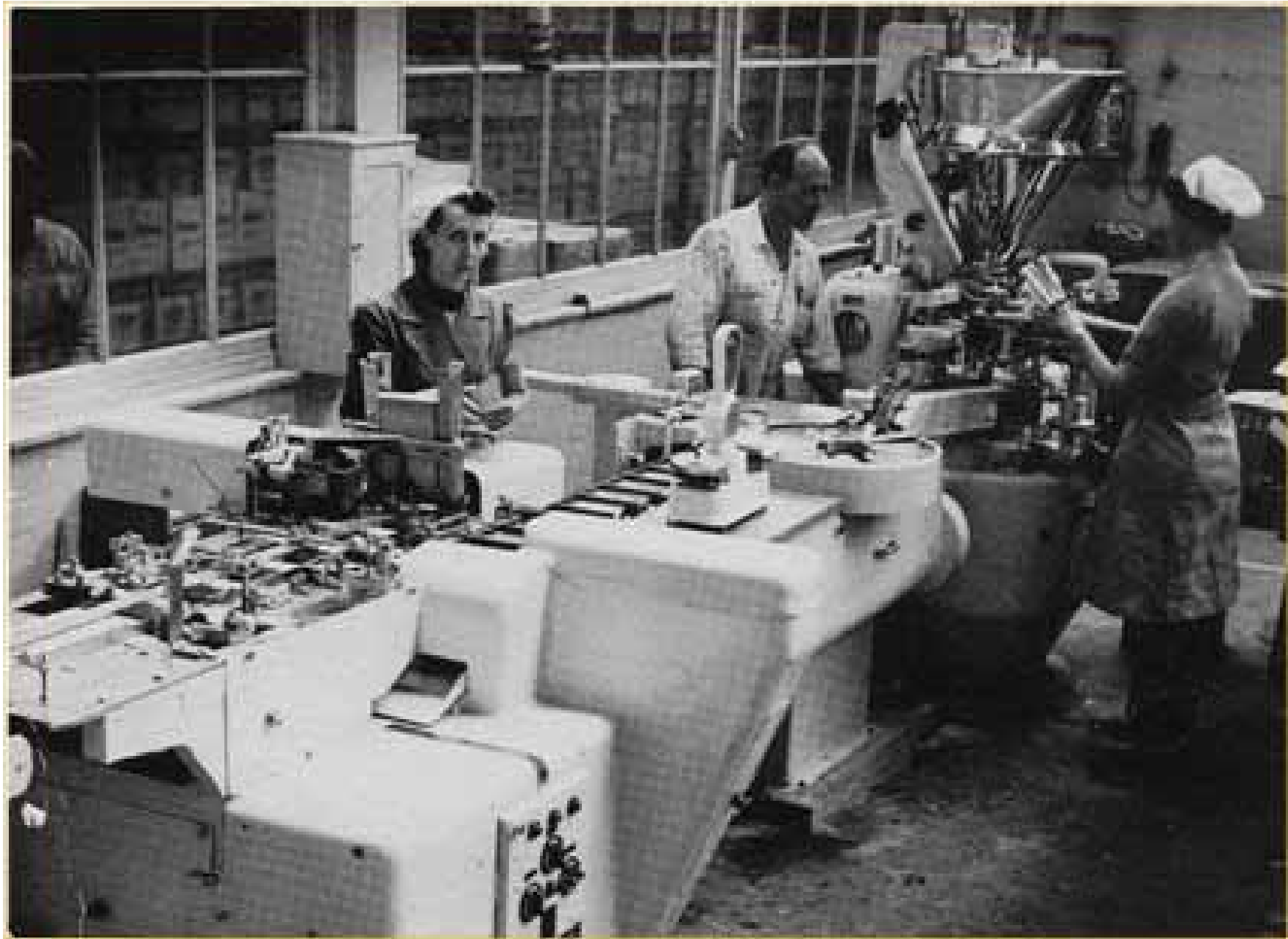
Toothpaste Balmain 1957 – first automated filler
